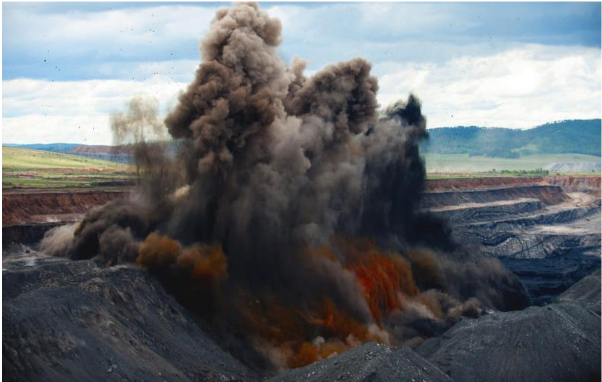
Figure 13: Typical Example of Dangerous Gas -Noxious Fume
